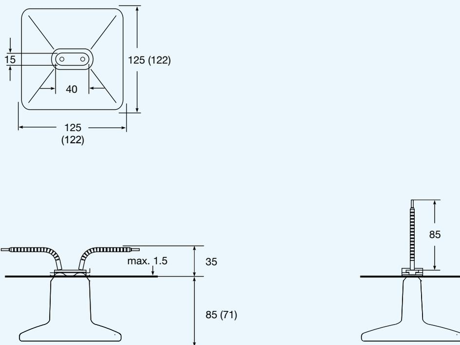
Figure 2: Mounting dimensions and radiator dimensions ( ) in mm
