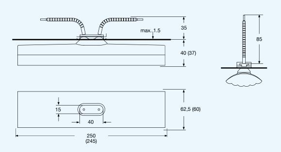
Figure 2: Mounting dimensions and radiator dimensions () in mm
